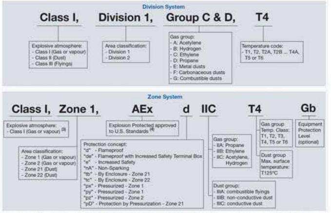
For Dust environments (Zone 21 or 22) the Class of the hazard (Class II) shall not be mentioned in the marking e.g. Zone 21, AEx to IIIC T125°C Ob
